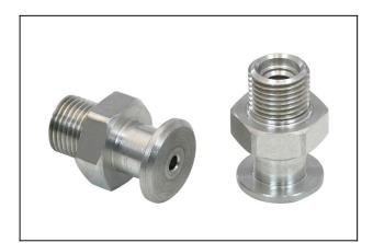
Nipple: N 008 Thread G1: G1/8"-M Overall length: 22 mm Fitting length: 5 mm Nominal size: 2,40 mm Material: Aluminium
