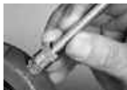
3. Seal and tighten Zerk-Lock using a hammer and staking tool
