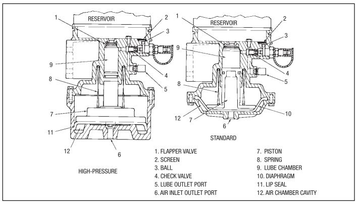
Figure 3. Air-Operated Pump Operation
