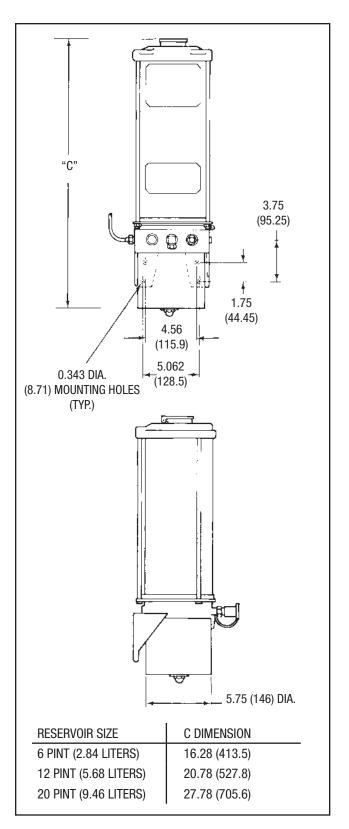
Figure 10. Electric Motor Pump - Dimensions
