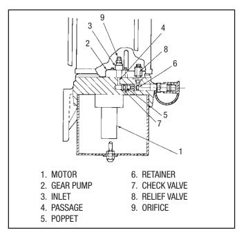
Figure 9. Electric Motor Pump Operation
