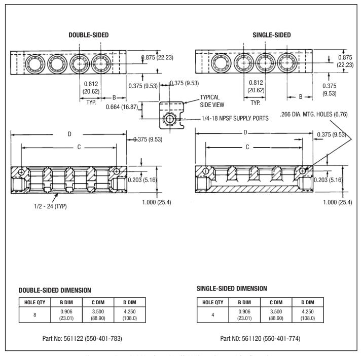
Figure 15. Extruded Aluminum Manifold Dimensions and Configurations
