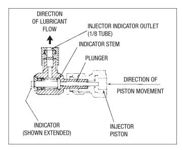
Figure 13. Injector Cycle Indicator Part No: 563769 (550-401-261)
