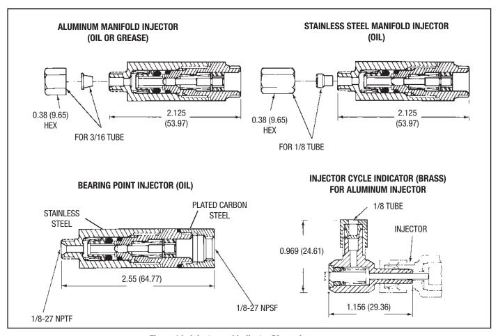
Figure 14. Injector and Indicator Dimensions
