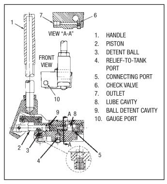
Figure 6. Hand-Operated Pump - Operation (Full upright position shown)
