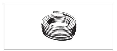
Figure 17. Tubing (unplasticized nylon)
