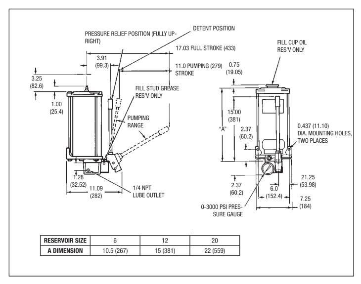
Figure 7. Hand-Operated Pump - Dimensions
