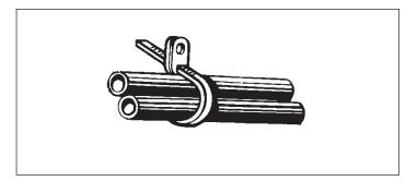
Figure 20. Tubing Straps
