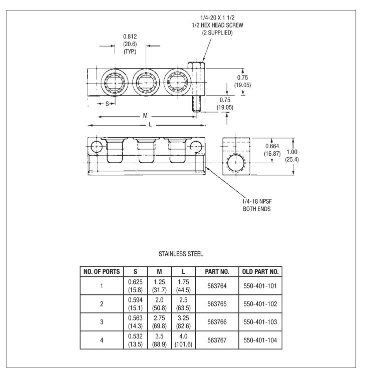
Figure 16. Stainless Steel Manifold Dimensions and Configurations
