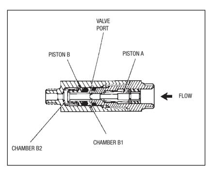
Figure 12. Injector Operation
