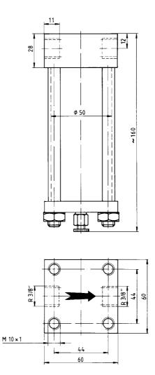
Assembly position as drawn. Space for dismounting of container and draining of condensate (screw 1) has to be available.
